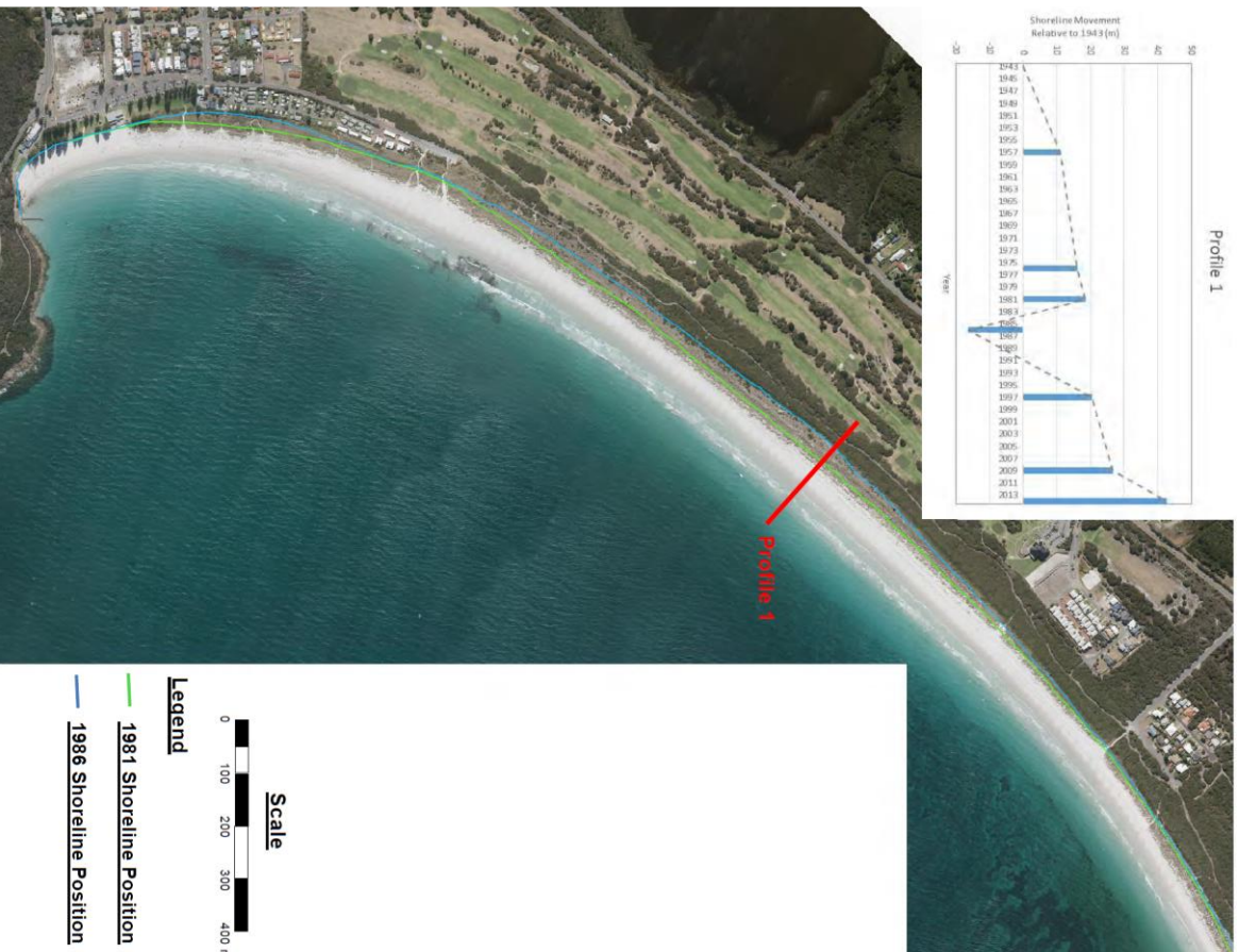
Figure 1 Extent of Erosion Along Middleton Beach Caused by 1984 Storm
