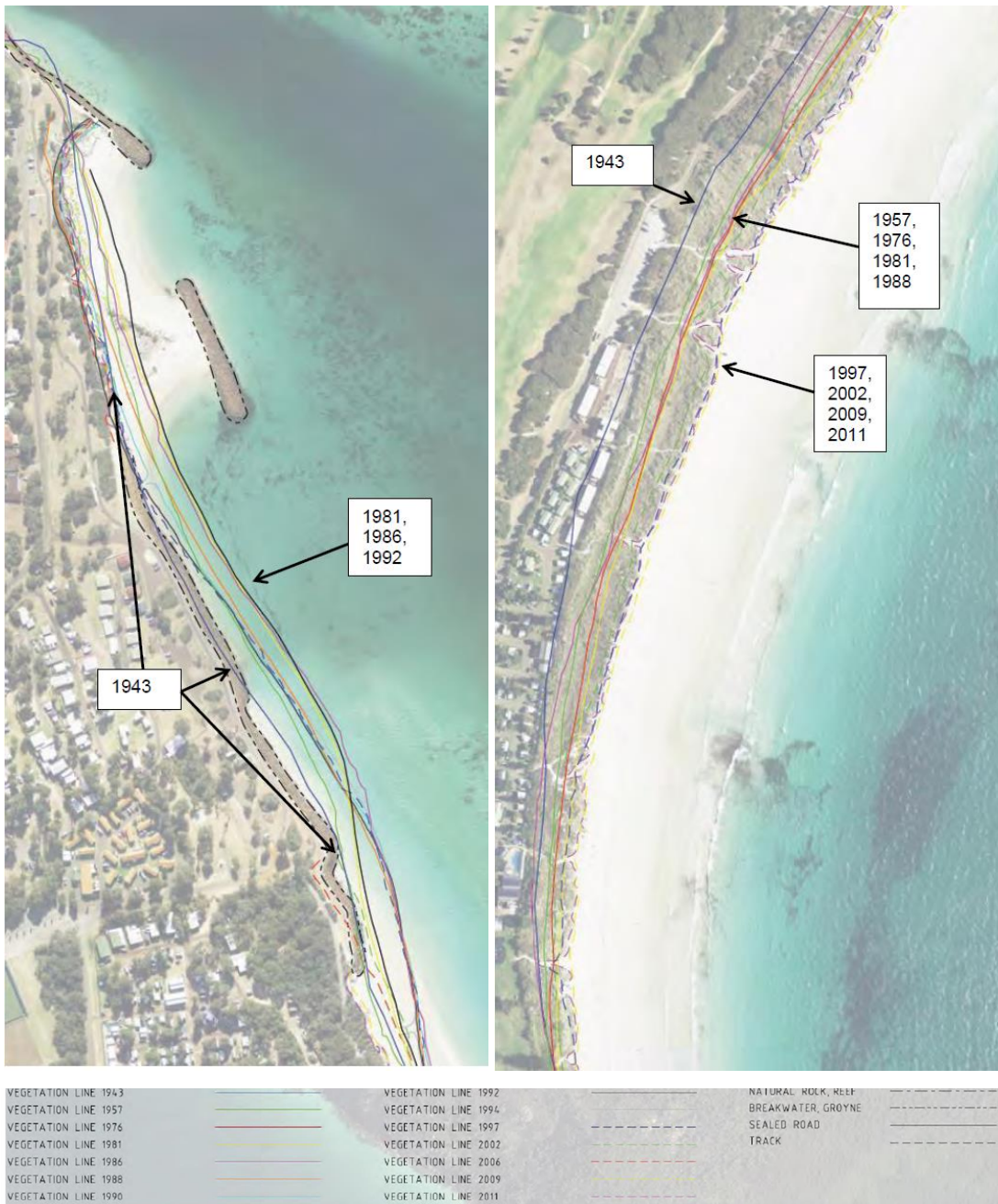
Figure B1-1 Analysis of aerial photography using vegetation lines to identify areas of erosion and accretion (source: DoT, 2012)
