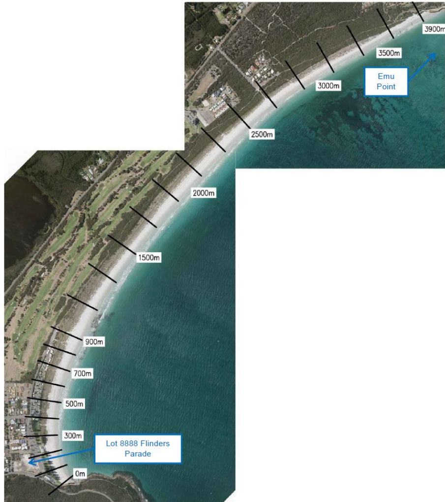
Figure B1-2 Chainage of shorenormal profiles used in interpretation of aerial photographs (source MP Rodger, 2015)
