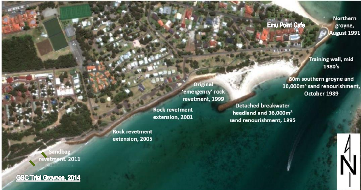
Figure 5 History of construction of coastal structures at Emu Point (source: PRDW, 2013a)
