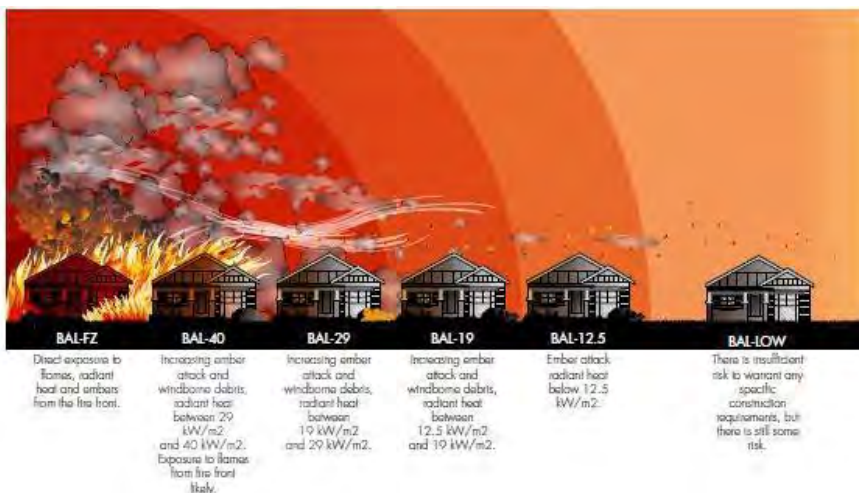
Figure 4: Building to BAL
