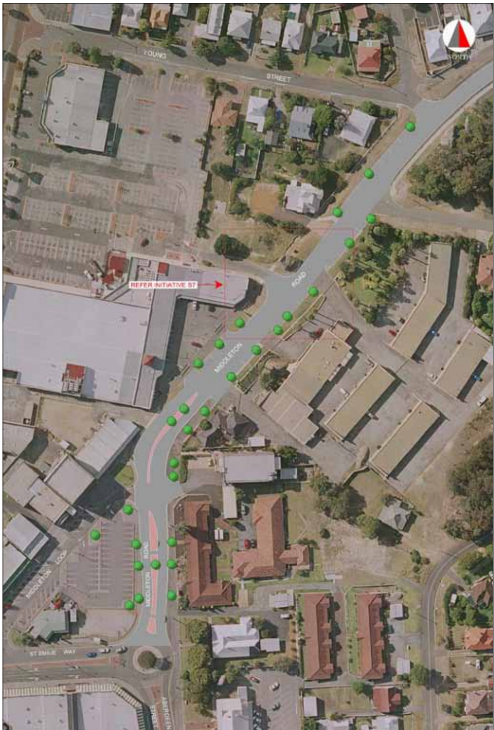
FIGURE 25 INITIATIVE S6 – Proposed Conceptual Streetscape Improvements & Provision of Embayed Kerbside Parking, Middleton Road
