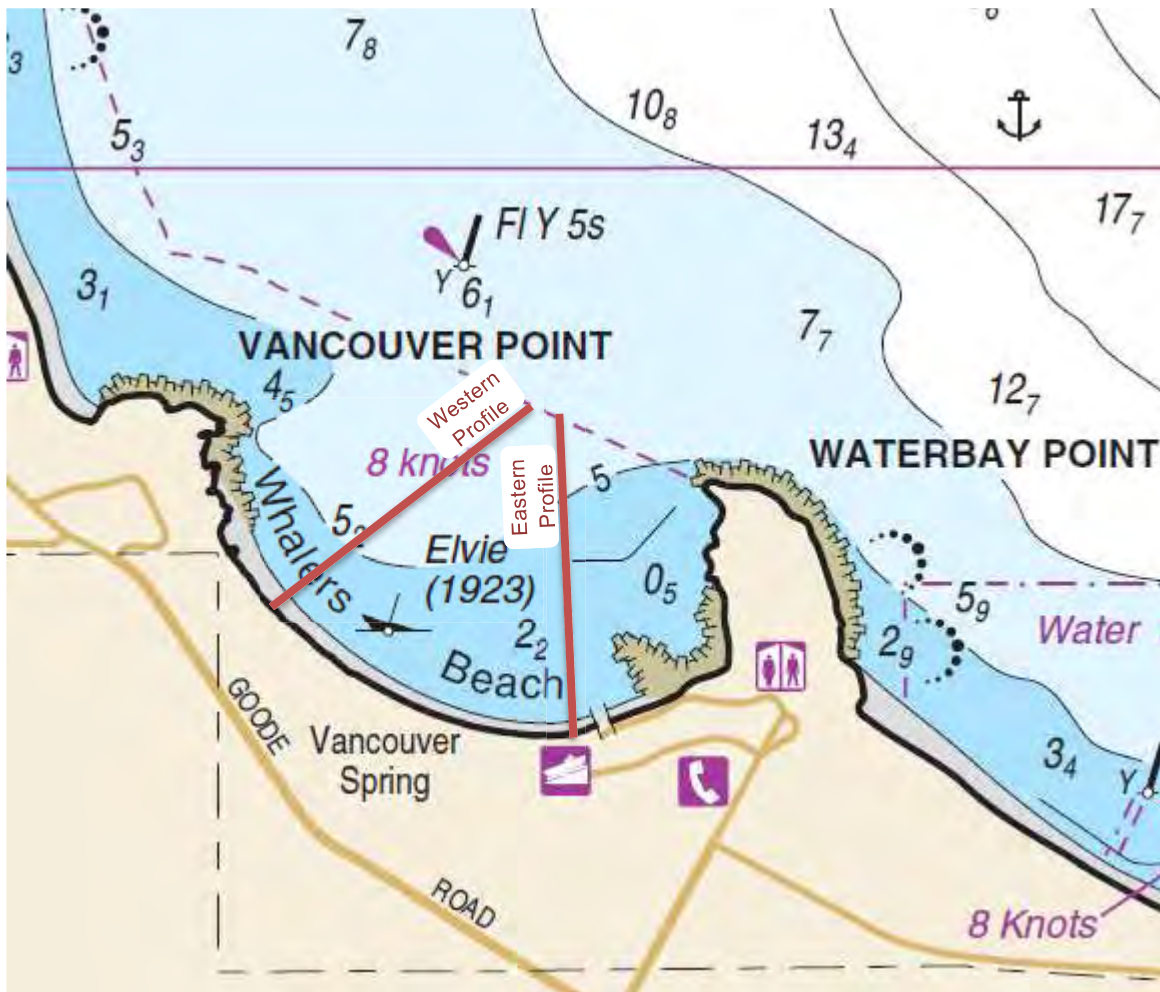
Figure 3.5 SBEACH Profile Location & Alignment
